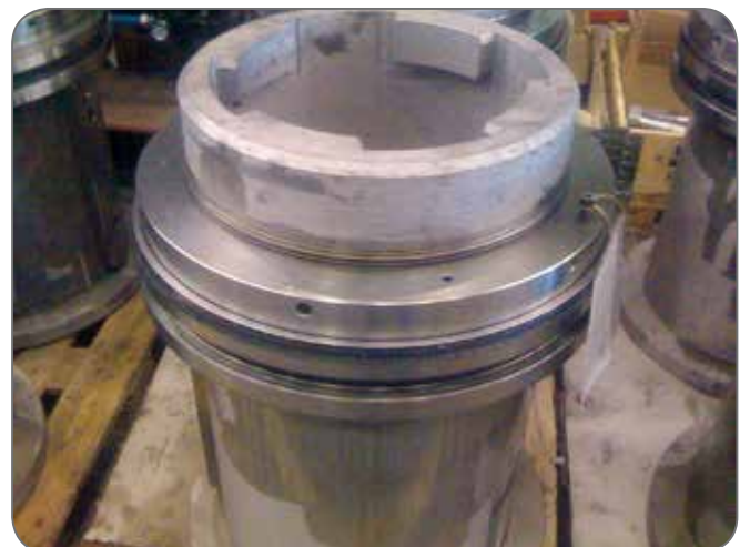
Hydraulic nut for propeller shaft-rudder coupling.
